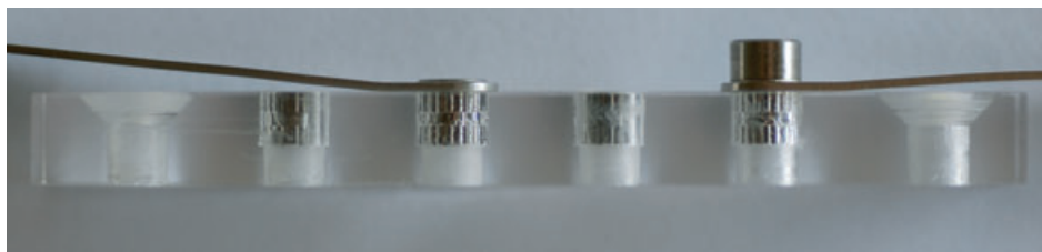
Fig. 3. Surgical guide with sleeves 3 mm from bone. At left 5 mm and at right 8 mm hand hold sleeve insert (drill key).
